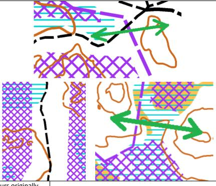
In the base material, the contours originally included 5 m contours and 2.5 m form lines (see picture on the right, the left part).
